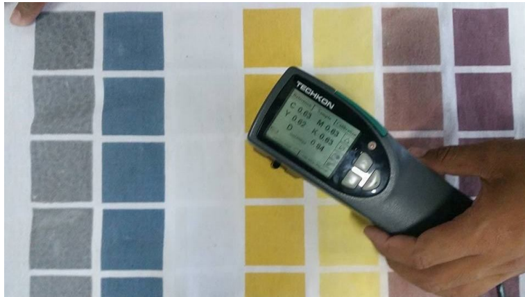
Figure 1 Measuring the values of density and L*a*b*of inks made from natural mordant and colorants
