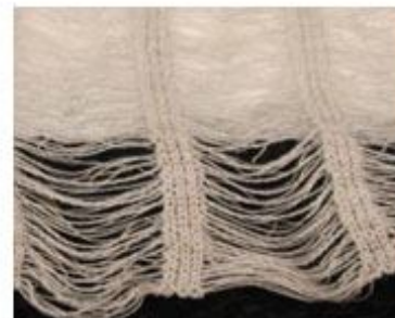
Fig. 2-6 Dropped loop structure
