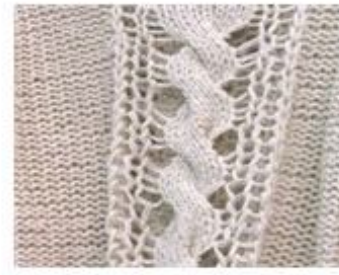
Fig. 2-3 Loop transfer coordinates knockover
